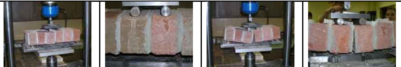
Four-Point Bending Test
